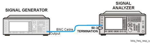
Figure 9-4. BBIQ Input Frequency Response Setup  $(\overline{Q} \text{ Input})$
