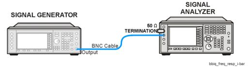
Figure 9-3. BBIQ Input Frequency Response Setup (Q Input)
