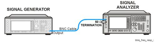
Figure 9-2. BBIQ Input Frequency Response Setup (I Input)
